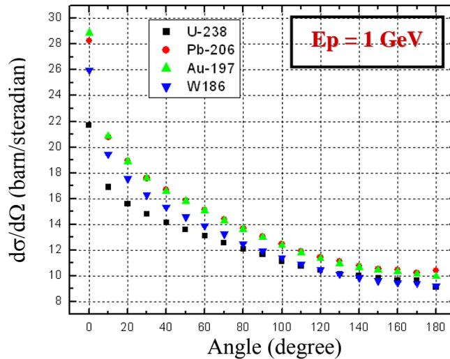
*Fig.5: Neutron angular distribution from 1 GeV proton induced reaction on  $^{238}\text{U}$ ,  $^{206}\text{Pb}$ ,  $^{197}\text{Au}$ ,  $^{186}\text{W}$*
