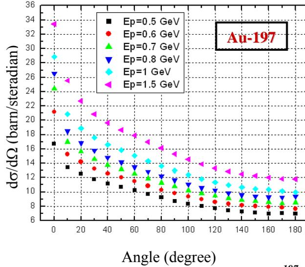
**Fig.8: Angular distribution of neutron on  $^{197}\text{Au}$  target with incident proton energies**
