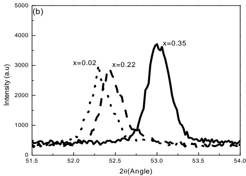
Figure 2(b): Position of the [116/312] diffraction peaks of single-phase  $\text{CuIn}_{1-x}\text{Ga}_x\text{Se}_2$  as function of gallium concentration ( $x=0.02, 0.22$  and  $0.35$ ).
