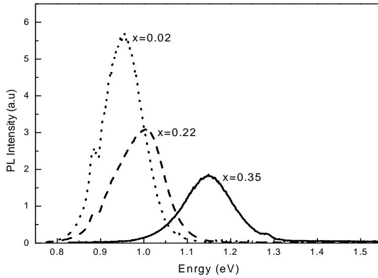
Figure 3: PL spectra for  $\text{CuIn}_{1-x}\text{Ga}_x\text{Se}_2$  samples selenized at  $550\text{ }^\circ\text{C}$  for 60 min, for different gallium concentration ( $x=0.02, 0.22$  and  $0.35$ ). Measurements were conducted at  $77\text{K}$ , using a  $5\text{mW}$  laser at an excitation wavelength of  $514.5\text{ nm}$ . The increase of the broadband peak position with increasing gallium content (increase in  $x$ ) is observed.
