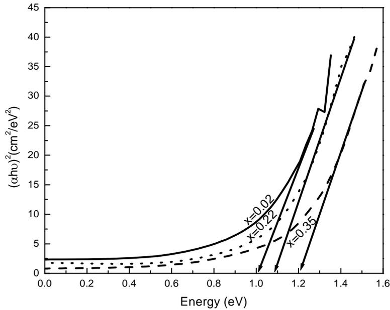
Figure 4: Graph of  $(\alpha h\nu)^2$  vs  $h\nu$  for different concentrations of gallium in  $\text{CuIn}_{1-x}\text{Ga}_x\text{Se}_2$  absorbers.
