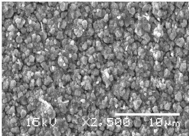
Figure 1(b): SEM micrographs showing the morphological features of a fully reacted  $\text{Cu(In,Ga)Se}_2$  film. Selenization was conducted in elemental Se vapour at 550 °C for 60 min.
