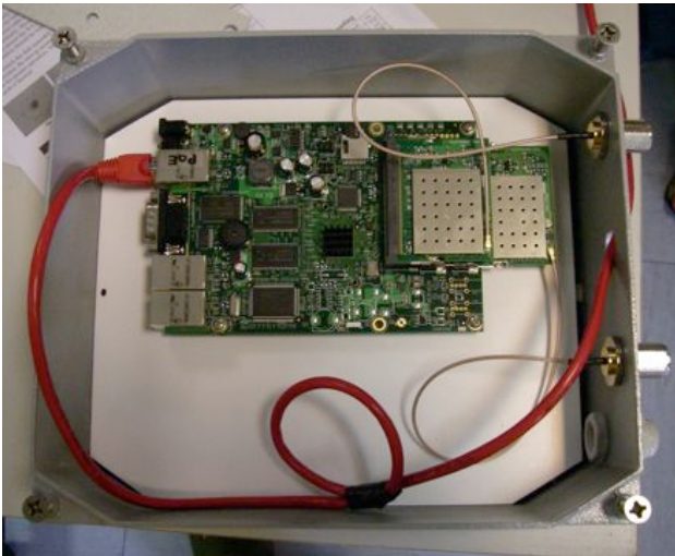
Figure 2. Mikrotik 433H wireless router fitted with two XR5 radios inside the weather proof housing. Notice the pigtailed for connection to the external antennas and the UTP cable that provides also PoE.
