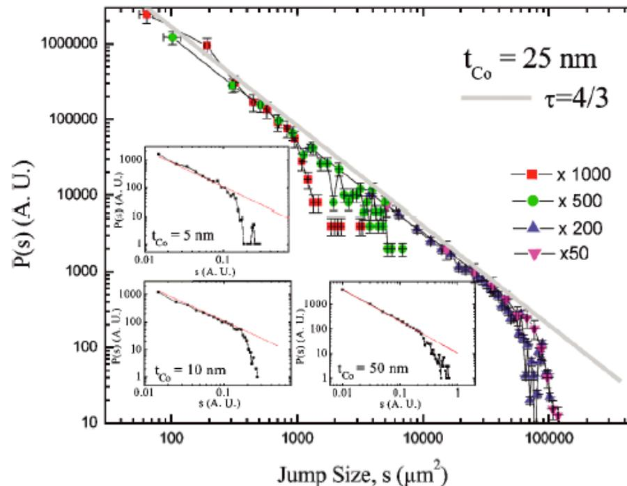
FIG. 3 (color). Distributions of the Barkhausen jump size in 25 and 50-nm Co samples. Distributions in 5, 10, and 50-nm Co samples are shown in the insets. Fitting curve with  $\tau = 1.33$  is denoted at each graph.
