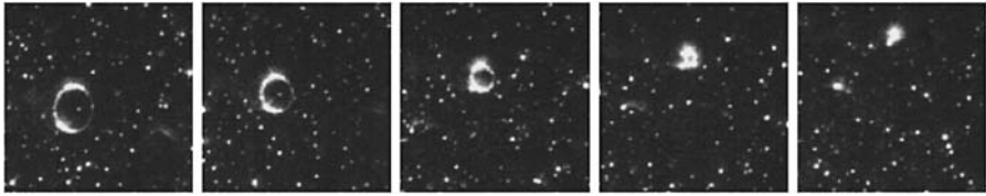
Fig. 1 The photos are taken 1 s apart, as a ring vortex ring passes through the sheet of illuminating light. The vortex is made visible by a collection of hydrogen particles that are trapped on its core. The width of each photo is 2 mm
