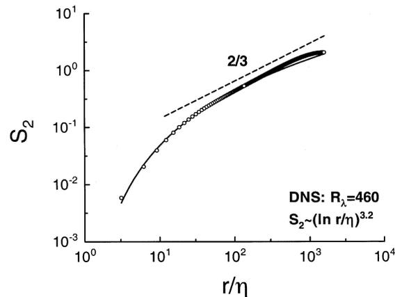
Figure 3. The second-order structure function  $S_2(r/\eta)$  against  $r/\eta$ . The DNS data [9] ( $R_\lambda = 460$ ) are shown as circles. The solid curve is the best fit of (3) corresponding to the logarithmic scaling. The dashed straight line is the Kolmogorov's 2/3rds scaling form, nominally thought to be applicable in the inertial range (ignoring effects of small-scale intermittency).
