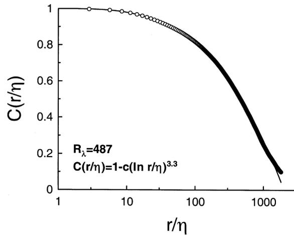
**Figure 9.** Correlation function for velocity fluctuations against  $r/\eta$  for  $R_\lambda = 487$  (circles). The solid curve is drawn in the figure to indicate agreement with the logarithmic scaling shown in figure 2.
