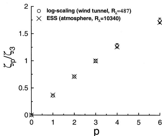
**Figure 5.** Normalized exponents  $\zeta_p/\zeta_3$  against  $p$  for  $R_\lambda = 487$  (circles). Crosses are the ESS exponents obtained for the atmospheric turbulence data at  $R_\lambda = 10,340$  [10].
