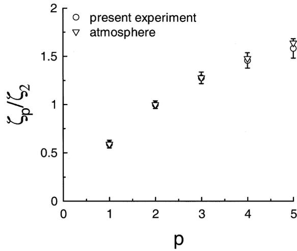
**Figure 8.** Exponents for the passive scalar extracted from figures 6 and 7 (circles) and for the fully developed atmospheric turbulence (ordinary scaling in the inertial range, triangles [12]).
