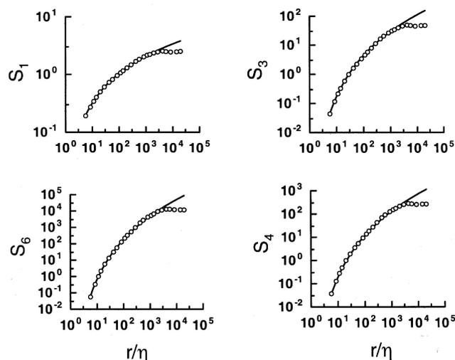
**Figure 4.** Structure functions of different orders ( $p = 1, 3, 4$  and  $6$ ) for  $R_\lambda = 487$  (cf. figure 2). The solid curves are drawn to indicate the logarithmic scaling (3).
