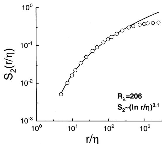
**Figure 1.** The second-order structure function  $S_2(r/\eta)$  against  $r/\eta$ . The experimental data ( $R_\lambda = 206$ ) are shown as circles. The solid curve is the best fit of (3) to the data, corresponding to the logarithmic scaling.
