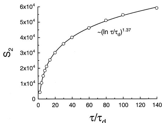
Figure 6. Second-order structure function of the temperature fluctuations for the heated wake.
