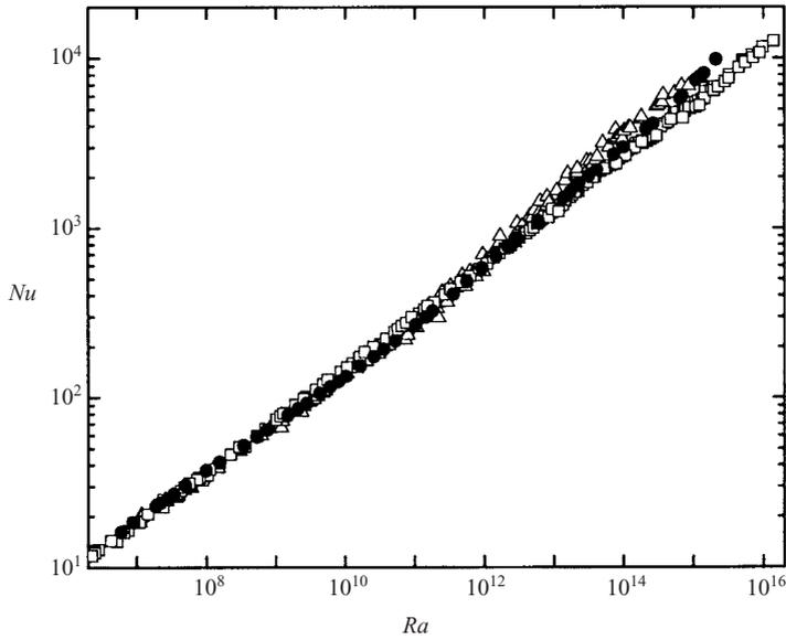
FIGURE 3. The variation of Nusselt number with Rayleigh number in log-log coordinates, from I ( $\square$ ) and II ( $\triangle$ ), compared with the present data ( $\bullet$ ). Only data determined to be 'nominally' Boussinesq by the various authors are shown. For all sets of data, this nominal criterion corresponds roughly to  $\alpha\Delta T < 0.2$ . We shall examine the adequacy of this criterion in §6.1 and Appendix C.
