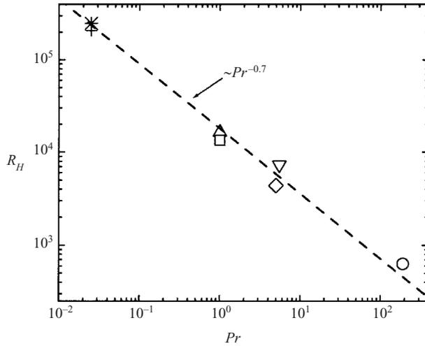
FIGURE 17. The variation of the bulk Reynolds number  $R_H$ , for  $Ra$  held fixed at  $10^{10}$ , versus  $Pr$  from various sources of data:  $\square$ , I;  $\triangle$ , II;  $\circ$ , Ashzenazi & Steinberg 1999, extrapolated;  $\nabla$ , Xin *et al.* 1996;  $\diamond$ , Sano *et al.* 1989;  $+$ , Cioni *et al.* (1997), extrapolated;  $*$ , Takeshita *et al.* (1996), extrapolated. The line marks  $R_H \approx 1.8 \times 10^4 Pr^{-0.7}$ .
