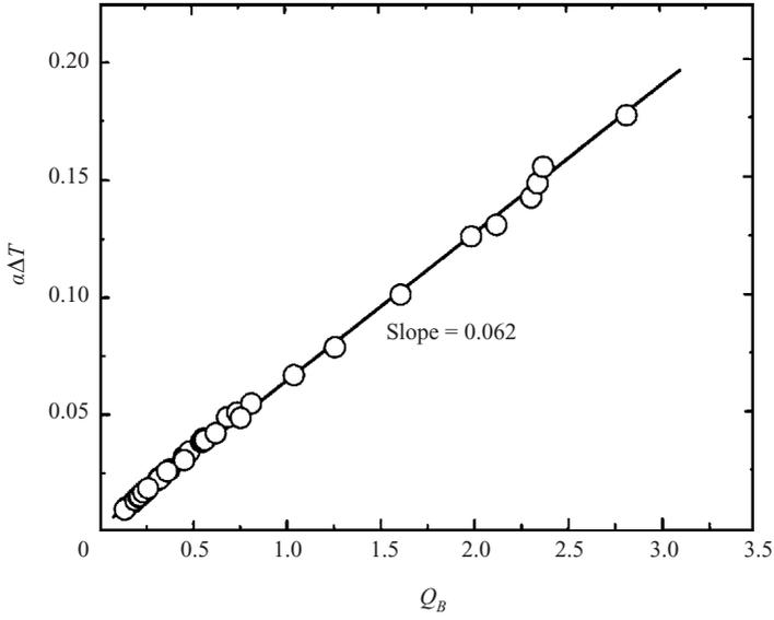
FIGURE 15.  $\alpha\Delta T$  as a function of the Boussinesq parameter  $Q_B$  defined by Busse (1967) for the present data. A linear relation holds with slope 0.062.
