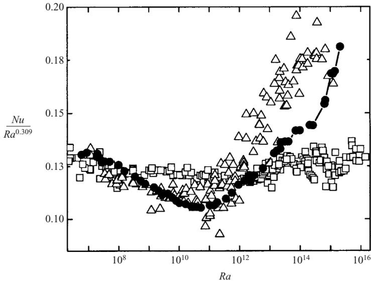
FIGURE 4. The Nusselt number data normalized by the 0.309 power of  $Ra$  for the same data as in figure 3. The present data ( $\bullet$ ) are similar to II ( $\triangle$ ) for low  $Ra$  but fall roughly intermediate between I ( $\square$ ) and II for high  $Ra$ . As in figure 3, only the data for which nominal Boussinesq conditions hold have been plotted.
