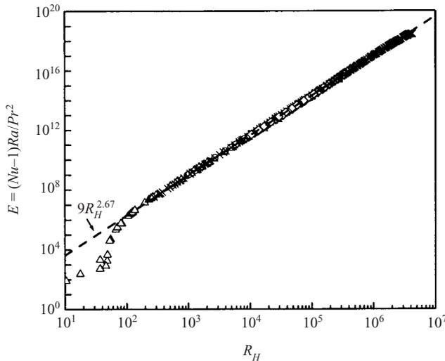
FIGURE 18. The dimensionless dissipation  $(Nu - 1)Ra/Pr^2$  as a function of  $R_H = 0.2Ra^{0.49}Pr^{-0.7}$ . The average dissipation is given to good approximation by the line  $9R_H^{2.67}$  over a large range of values.  $\triangle$ , II;  $\circ$ , present data;  $\times$ , I;  $*$ ,  $Pr = 0.7$ , Roche (2001);  $\nabla$ ,  $Pr = 1.5$ , Roche (2001);  $\diamond$ ,  $Pr = 1.1$ , Roche (2001).
