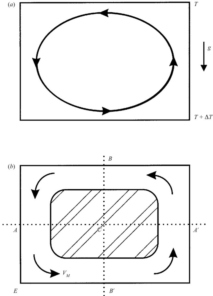
FIGURE 12. Schematic of (a) the mean wind at high Rayleigh numbers and (b) the idealized problem solved by numerical simulations. The hatched region is assumed not to participate in the flow. The rounding of the corners has been varied by a factor of two with no perceptible changes in the heat transport results.
