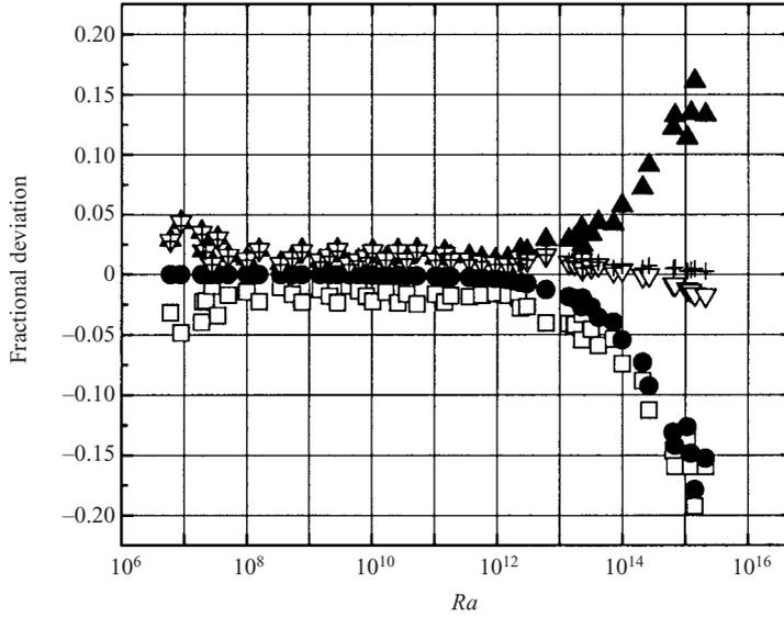
FIGURE 6. The fractional deviation about the mean of various fluid properties for the present data: ●, specific heat,  $C_P$ ; +, kinematic viscosity,  $\nu$ ; □, thermal expansion coefficient,  $\alpha$ ; ▲, thermal diffusivity,  $\kappa$ ; ▽, thermal conductivity,  $k_F$ . These quantities vary by less than 5% for  $Ra$  up to  $10^{14}$ , but some of them vary by as much as 20% by  $Ra = 10^{15}$ .
