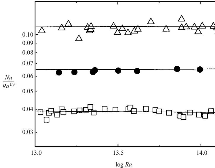
FIGURE 10. Data beyond the dotted line in figure 9 have been expanded here, showing more clearly the  $1/3$  scaling for the three data sets. As in figure 9, Nusselt numbers are normalized by  $Ra^{1/3}$  and displaced vertically by the same amounts as in figure 9.  $\square$ , I;  $\triangle$ , II;  $\bullet$ , the present data.
