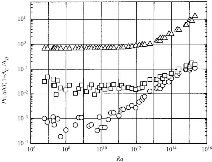
FIGURE 8. The Prandtl number ( $\Delta$ ) and the parameters  $\alpha\Delta T$  ( $\square$ ) and  $1 - \Delta_c/\Delta_H$  ( $\circ$ ), as functions of  $Ra$  in the present measurements.
