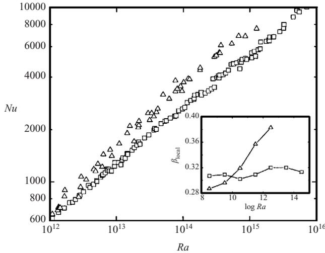
FIGURE 1. The variation of the Nusselt number with the Rayleigh number in log–log coordinates, from I ( $\square$ ) and II ( $\triangle$ ), illustrating the difference for  $Ra > 10^{12}$ . Inset shows approximate local slopes,  $\beta_{local} = d \log(Nu)/d \log(Ra)$ , obtained by least squares fits over running intervals of three decades. Various trials suggest that local slopes are less robust if shorter running intervals are used.
