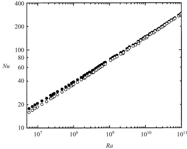
FIGURE 13. The Nusselt number data, obtained for the case of bare stainless steel walls bounding the fluid, corrected according to the results of numerical simulations. ●, Uncorrected  $Nu$ ; ○, corrected  $Nu$ . The correction is negligible beyond  $Ra$  of about  $10^9$ . The correction schemes devised by Ahlers (2000) are similar though the magnitudes are somewhat larger.
