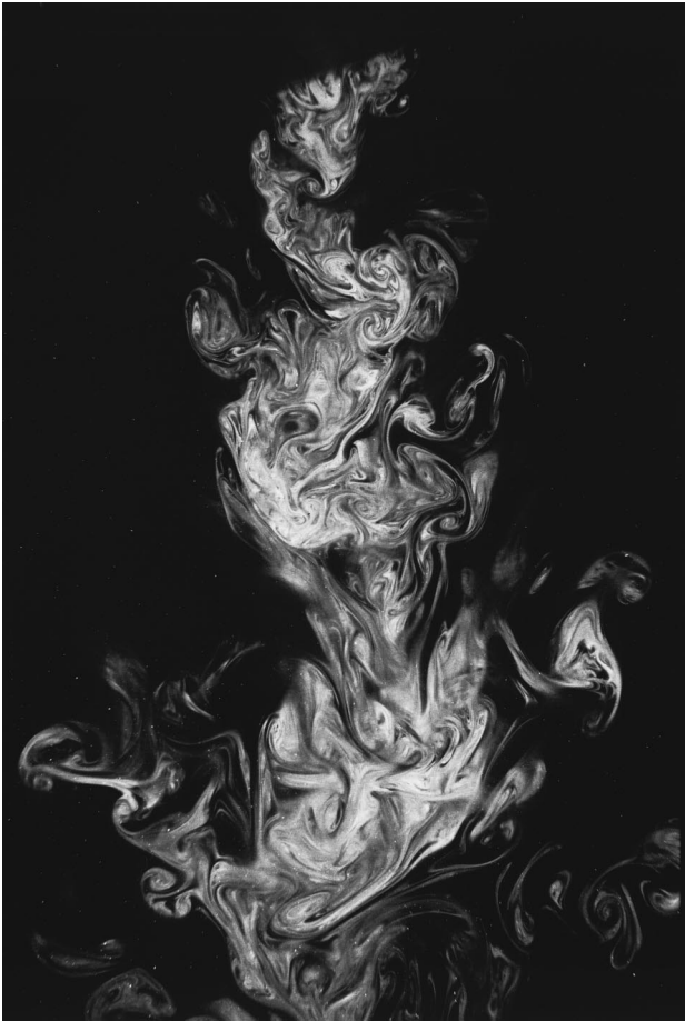
FIG. 1. A turbulent jet of water emerging from a circular orifice into a tank of still water. The fluid from the orifice is made visible by mixing small amounts of a fluorescing dye and illuminating it with a thin light sheet. The picture illustrates swirling structures of various sizes amidst an avalanche of complexity. The boundary between the turbulent flow and the ambient is usually rather sharp and convoluted on many scales. The object of study is often an ensemble average of many such realizations. Such averages obliterate most of the interesting aspects seen here, and produce a smooth object that grows linearly with distance downstream. Even in such smooth objects, the averages vary along the length and width of the flow, these variations being a measure of the spatial inhomogeneity of turbulence. The inhomogeneity is typically stronger along the smaller dimension (the “width”) of the flow. The fluid velocity measured at any point in the flow is an irregular function of time. The degree of order is not as apparent in time traces as in spatial cuts, and a range of intermediate scales behaves like fractional Brownian motion.
