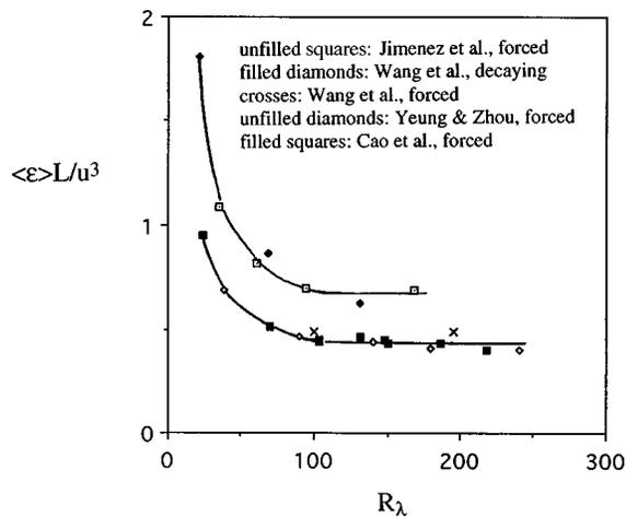
FIG. 1. The variation of the quantity  $\langle \epsilon \rangle L/u^3$  with the Taylor microscale Reynolds number,  $R_\lambda$ , in simulations of homogeneous and isotropic turbulence in periodic box. The symbols, described on the figure, correspond to different sources of data noted in Table I.
