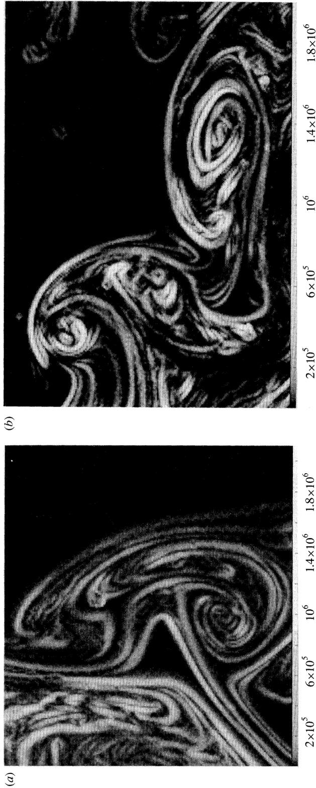
Figure 4. (a) Close-up of a typical spiral-like structure in a transverse section of the jet. (b) Similar close-up from a longitudinal section.
