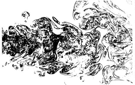
The small-scale structure of the scalar in a round jet of water at a nozzle Reynolds number of 4,000. From the concentration field of a dye obtained by laser-induced fluorescence (for details, see ref. 9), one constructs a two-dimensional graph of the square of the gradient of the concentration. This quantity represents the small-scale features of the scalar. The resolution of measurement is between one and two Kolmogorov scales. Much finer scales of the scalar have not been resolved.
