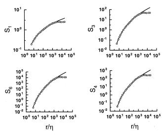
**Figure 4.** Structure functions of different orders (p = 1, 3, 4 and 6) for  $R_{\lambda} = 487$  (cf. figure 2). The solid curves are drawn to indicate the logarithmic scaling (3).
