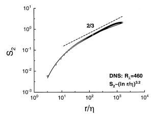
**Figure 3.** The second-order structure function  $S_2(r/\eta)$  against  $r/\eta$ . The DNS data [9] ( $R_{\lambda} = 460$ ) are shown as circles. The solid curve is the best fit of (3) corresponding to the logarithmic scaling. The dashed straight line is the Kolmogorov's 2/3rds scaling form, nominally thought to be applicable in the inertial range (ignoring effects of small-scale intermittency).
