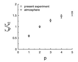
Figure 8. Exponents for the passive scalar extracted from figures 6 and 7 (circles) and for the fully developed atmospheric turbulence (ordinary scaling in the inertial range, triangles [12]).
