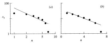
Figure 6. The log-log (a) and semi-log (b) plots of  $x_n$  against n for the spiral-like structures in a longitudinal jet section.
