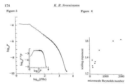
Figure 5. A typical spectral density of temperature fluctuations in the wake of a heated circular cylinder. The oncoming mean air speed was 1770 cm s<sup>-1</sup>, and the cylinder was 20 mm in diameter. Measurements were made approximately 100 diameters downstream of the cylinder on the wake centreline. At the measurement station, the root-mean-square temperature fluctuation was about 0.36 °C. The inset shows that the slope is close to  $\frac{4}{3}$  with about 1.5 decades of scaling.
