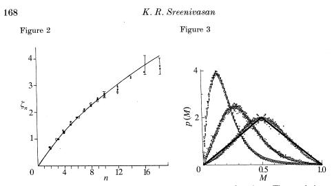
Figure 2. The scaling exponent  $\zeta_n$  for the velocity structure functions. The symbols are for a turbulent duct flow and a jet, from Anselmet *et al.* (1984). The continuous line is from Chhabra & Sreenivasan (1991b) for the atmospheric turbulence.
