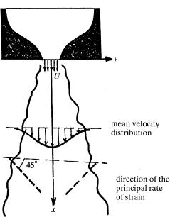
Figure 1. Schematic of a turbulent jet (for example, water jet flowing into water) and the coordinate axes. The outer boundary roughly reflects the average growth of the jet. Typical mean velocity distribution and directions of the principal strain rates in the jet are shown.
