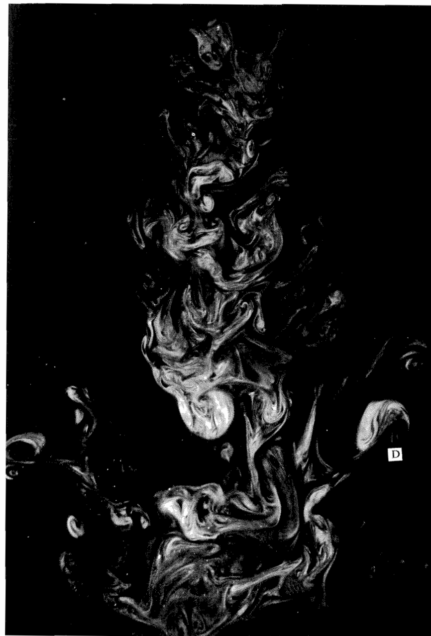
FIGURE 2. A two-dimensional slice of a turbulent jet at a nozzle Reynolds number of about 4000, obtained by the LIF technique. The entire extent of the CCD array ( 1300 \times 1000 pixels) was used to obtain this image. The region imaged extends from 8 to 24 diameters downstream of the nozzle. A Nd:YAG laser beam shaped into a sheet of about 250 \mu\text{m} thickness using a suitable lens was directed into the water tank into which the nozzle fluid containing small amounts of a fluorescing dye was emerging in the form of a jet. The laser had a power density of 2 \times 10^7 \text{ J s}^{-1} per pulse and a pulse duration of about 10 ns.
