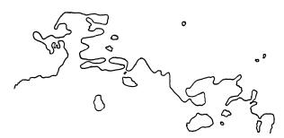
FIGURE 5. Planar intersection of the surface with the mixture fraction 0.5 in a fairly low Reynolds number turbulent mixing layer.
