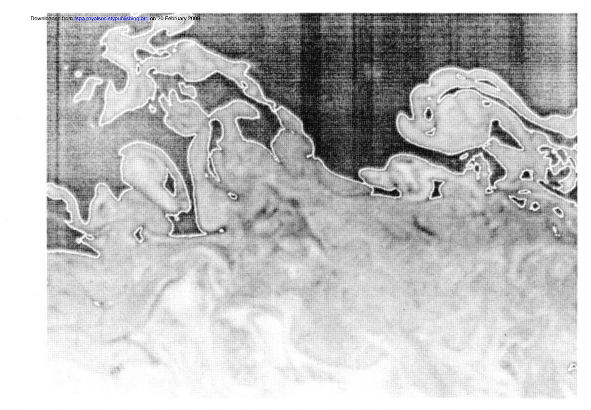
'IGURE 11. Section of a countercurrent flow at a moderate Reynolds number, obtained by using laser-induced fluorescence. Also shown as the white line is the interface drawn by setting a suitable threshold to demarcate the bright regions from the dark.
