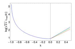
Fig. D.11. Maximal eigenvalue  $\log \lambda_{\max}(k)$  computed for truncated matrices O(k) with basis sets of size L = 120 (red), L = 200 (green), L = 300 (blue). Close to the singularity k = -1,  $\lambda_{\max}(k)$  converges rapidly with L. (For interpretation of the references to color in this figure legend, the reader is referred to the web version of this article.)
