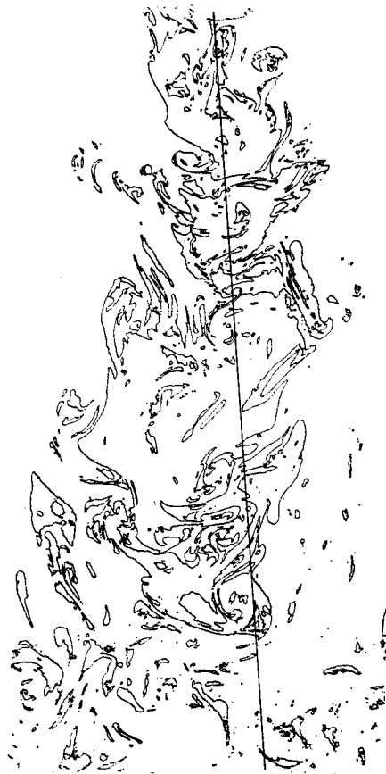
Figure 7 The boundary of a jet in a two-dimensional intersection, and its intersection with a line in the plane of the two-dimensional section. The points of intersection form a set whose dimension can be calculated by box counting. Sreenivasan et al (1989a) have calculated the dimension as a function of the vertical and horizontal positions, as well as the orientation, of line cuts, and they found the dimension to be consistently the same.
