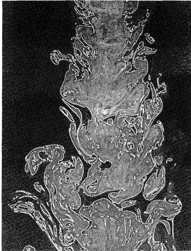
Figure 4 The two-dimensional image of Figure 3, with the computer-generated boundary representing the interface between the scalar-marked region and the ambient unmarked fluid in the tank. The boundary was generated by setting a threshold on the pixel intensity in the digital image. The boundary is generally realistic, but (since some minor ambiguities do remain) sensitivity checks are essential; see Figure 5 (from Prasad & Sreenivasan 1990b).
