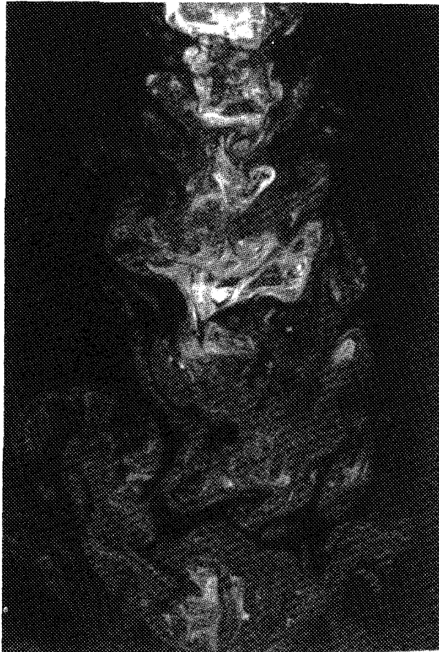
Figure 3 A two-dimensional image of an axisymmetric water jet, obtained by the laser-induced fluorescence (LIF) technique. A Nd:YAG laser beam shaped into a sheet of 200–250 \mu\text{m} thickness using suitable lenses was directed into a water tank into which the jet fluid was emerging from a well-contoured nozzle and standard upstream flow management; the jet fluid contained small amounts of uniformly dispersed fluorescing dye (sodium fluorescein). The fluorescence excited by the laser radiation was captured on a digital camera (a charge-coupled device, with a pixel array size of 1300 \times 1035 ). The pixel intensity in the digital image was linearly related to the concentration of the dye. Different shades of gray in the figure qualitatively reflect different concentration levels. The laser had a power density of about 2 \times 10^7 \text{ J s}^{-1} per pulse and a pulse duration of 10 ns. The flow is thus frozen to an excellent approximation. The region in the image extends from 8 to 24 nozzle diameters. The nozzle Reynolds number was about 4000. The laser-sheet thickness was between \langle \eta \rangle and 2\langle \eta \rangle , where \langle \eta \rangle is the Kolmogorov thickness averaged over the image (from Prasad & Sreenivasan 1990b).
