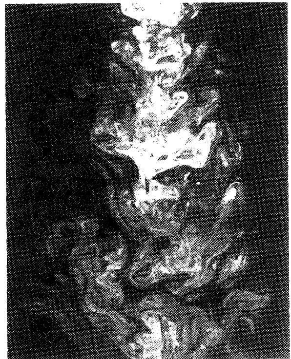
FIG. 1. Two-dimensional laser induced fluorescence image of an axisymmetric water jet. The region imaged extends from 8 to 24 diameters downstream of the nozzle. The nozzle Reynolds number is 4000. A discussion of relevant experimental techniques is given in Sec. II.
