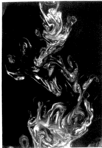
Fig. 6. Two-dimensional laser-induced fluorescence visualization of a plane section of the jet taken one diameter off-axis
