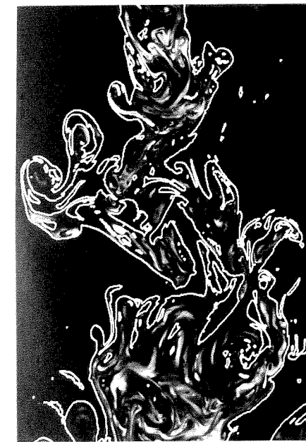
Fig. 9. Computer generated interface (marked white) of the jet section shown in Fig. 6; the interface was generated using the threshold found from the slope change of the thresholded average intensity curve of Fig. 8
