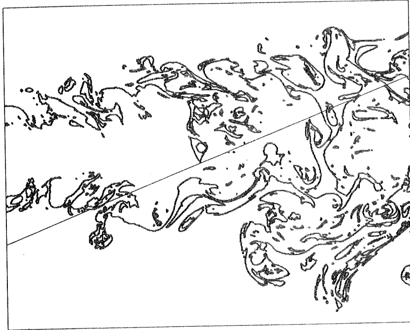
Figure 2. The boundary of the jet crosssection given in figure 1, determined by prescribing a threshold on brightness ( \sim the concentration of the nozzle fluid). Also shown is a typical line intersection of the boundary; this will be discussed later in the text
