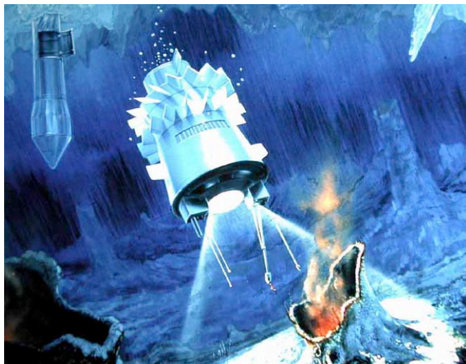
Fig. 2: The earlier hydrobot-cryobot proposal for directly probing Europa's ocean, Horvath et al , (1997), http://www.ictp.it/~chelaf/searching_for_ice.html
